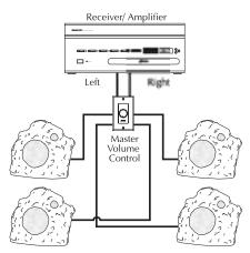
Figure 4 One Zone Volume Control Wiring
